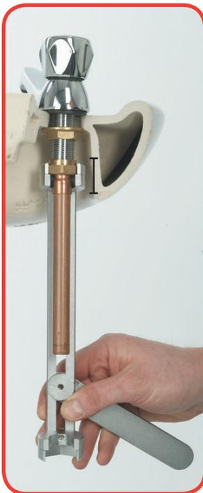
Sliding jaws locked in position to allow tightening / removal of pipe nut.
