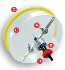
A 2 Adjustable HSS Cutting Blades Adjustable cutting blades can be altered to cut a variety of diameters from 40 – 203mm for the ultimate flexibility. Also reduces the need to carry a holesaw for every size, making it the cost effective solution to creating large diameter holes
