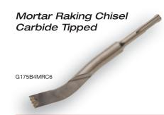
A cranked shaft chisel which is purpose designed to not "dive-in" to mortar lines, but effectively chisel away stubborn mortar. The cranked shaft allows for access behind down-pipes and close up to door and window frames for a neat finish without damage
